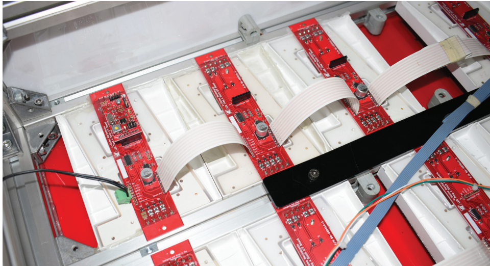
Figure 6. Wiring example of a Serial LED Display Unit in a installation. PFC and ribbon wire connectors are used to connect the modules together. This results in a easy and neat wiring installation.
