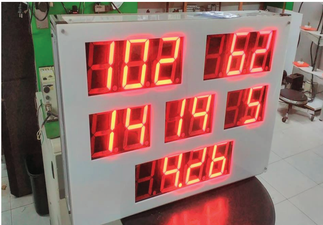
Figure 7. Sample Scoreboard project with Serial LED Display system. 16 panels or digits used.
