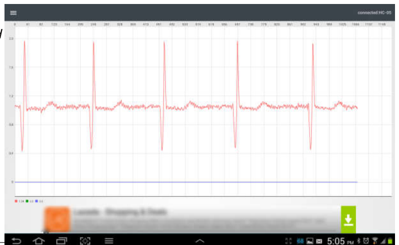
Figure 6. Clipping occurring in Fig.5 is eliminated by adjusting RV1.
