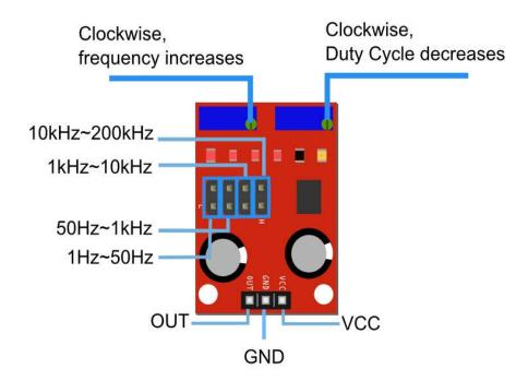
Figure 1. Pinouts of Pulse Frequency module.
