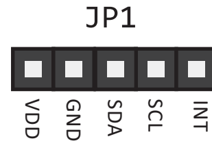
Figure 1. JP1 Pin I.D. Illustration
