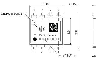
Acceleration in the direction of the arrow will increase the output voltage.
