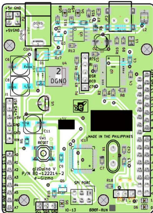
Figure 8. Bottom PCB layout guide
