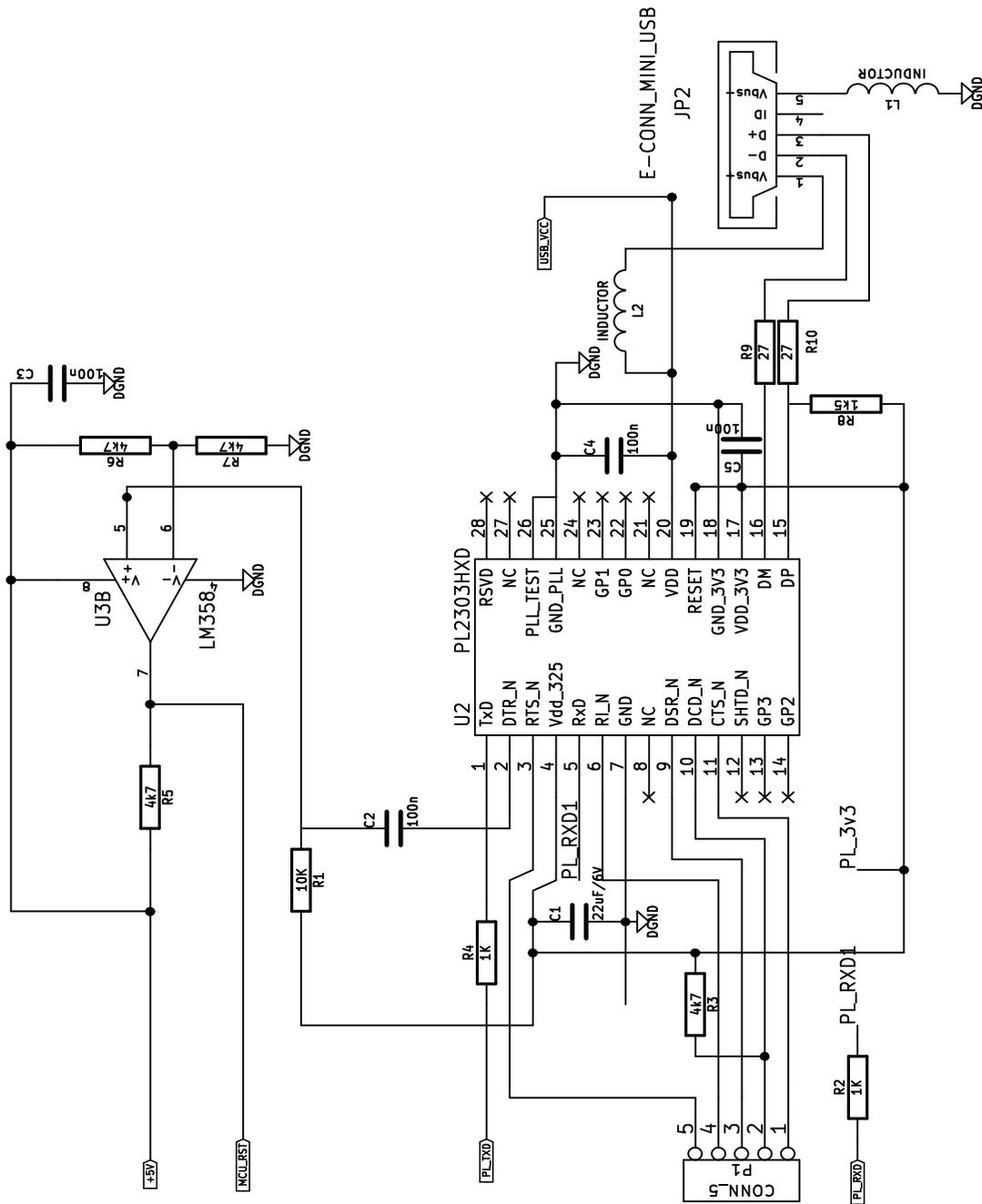
Figure 10. Schematic Diagram of e-Gizmo Prolific Driver PL2303.
