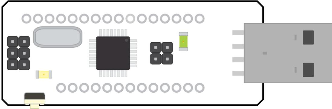
gizDuino mini variant with USBasp Loader firmware and USB programming port to form a complete low cost Arduino compatible mini board! No need for a separate USB programmer. Choice of ATMEGA328 or ATMEGA168 controller.
