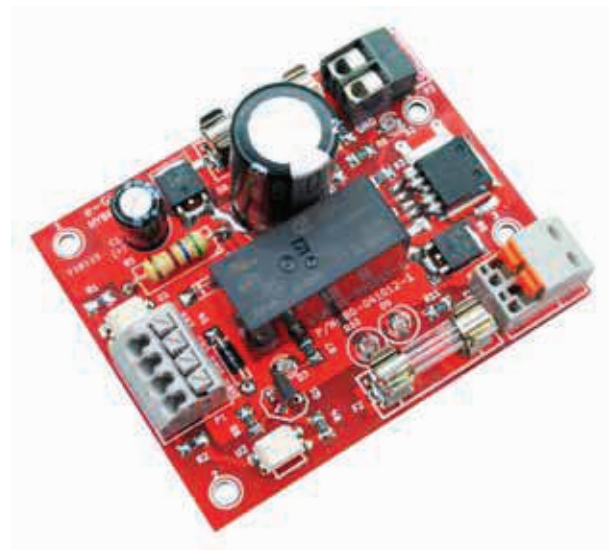
Figure 1. The DC Motor Hybrid Drive is available in 12V and 24V DC Version.
