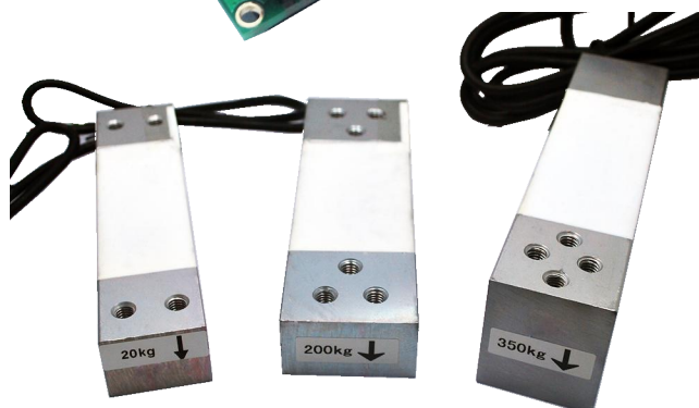
Figure 1. Loadcells Available 3kg to 400kg (*Optional)
