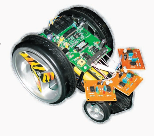
Figure 14. The Universal Programmable Robot Controller UPRC wired to do one of its favorite thing - MOBOT controller.
