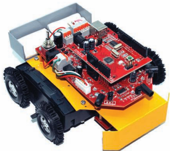
P-BOT Mobile Robot with gizDuino Controller installed.
