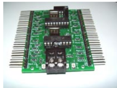
Figure 1.7. Motor power supply connector J17 and LED indicators.
