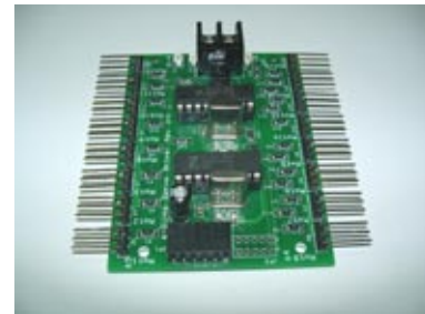
Figure 1.8. Host interface connector JP1 allows the host controller board to link directly with the servo driver-controller without the use of wires.
